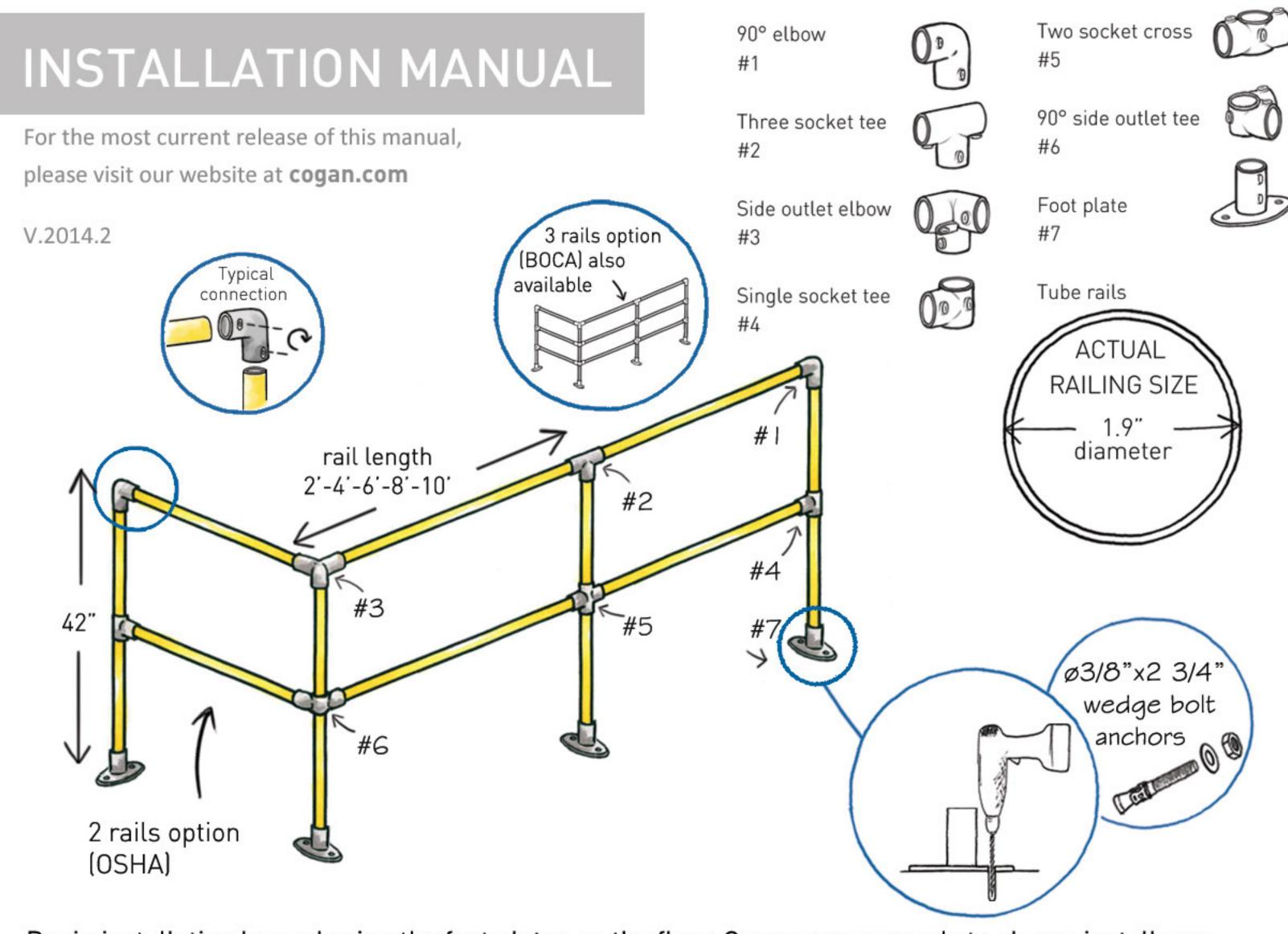
Begin installation by anchoring the foot plates on the floor. Cogan recommends to always install on a concrete surface. Refer to installation drawings for the layout.
